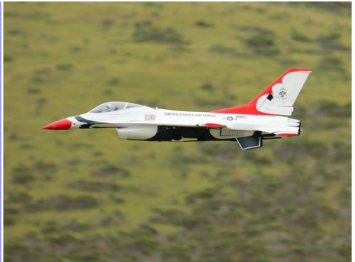
This is Harold's E-Flite F-16, 70mm fan on 6S battery, with retractable gears.
