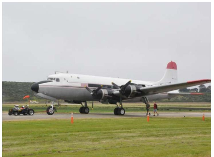
The largest plane, a Douglas DC-4. It is converted to spray oil dispersant fluid over the oil spills at sea.
