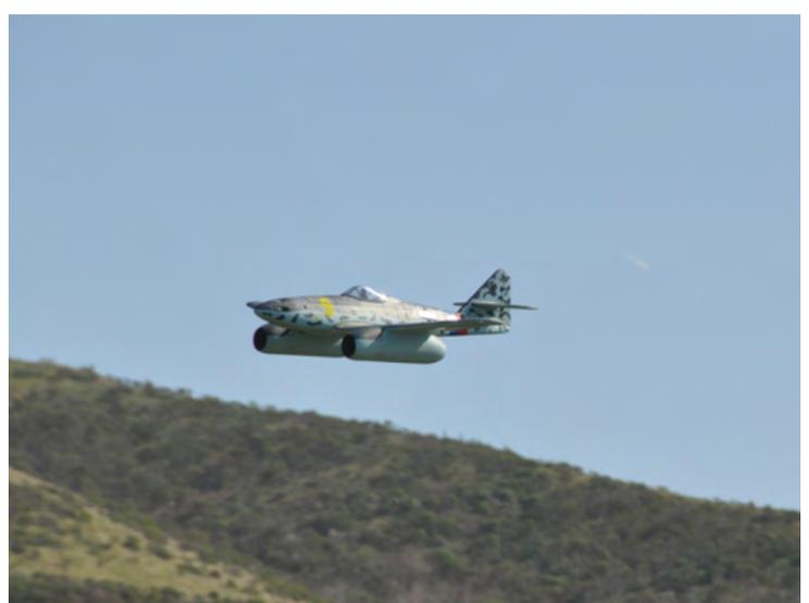
Martin's ME-262 on a low pass, twin ducted fans, retractable landing gears.
