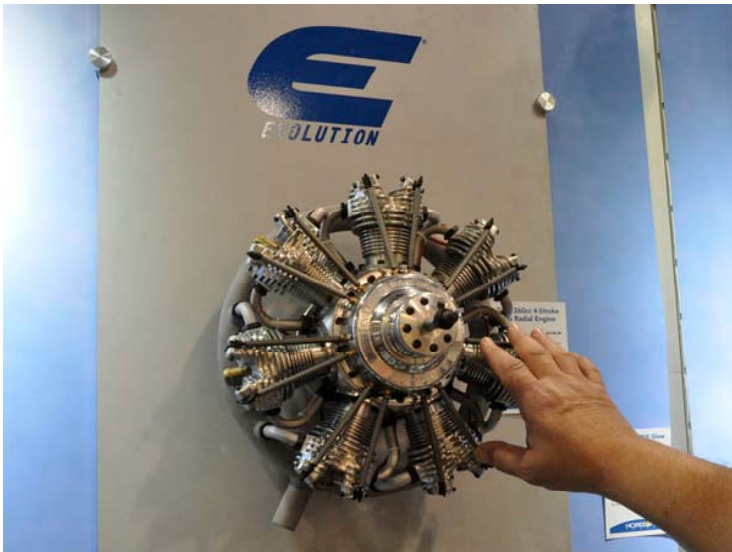
Evolution 7 Cyl 260 c.c. ignition engine. (buddy's hand for sizing.)
