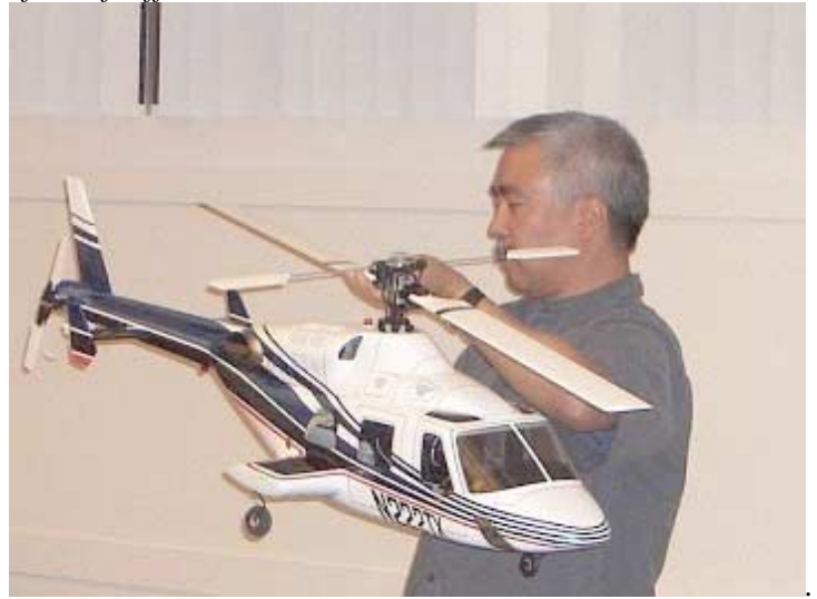
Dan Young's Raptor 50SE converted to electric in a Century Bell 222 fuselage.
