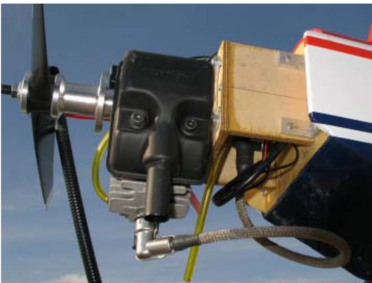
This is a view of the 20cc Zeonah showing the muffler.
